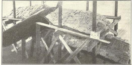
FAILURE OF AN AIRPLANE WING IN STATIC TESTING
