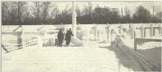
A VIEW IN FRONT OF THE PROPELLER RIG, AFTER A SIX-HOUR WATER-SPRAY TEST
